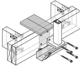
Gutter Brackets have been designed for easy attachment of standard New Zealand gutter systems. Available on Homestead®, Viking®, Edge® and Edgetec® Mini Post balustrade systems.
