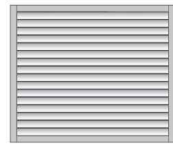
HORIZONTAL LOUVRE INFILL 58MM, 80MM, 120MM OR 150MM
